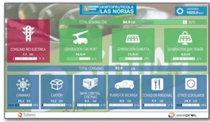
The integration of all the activities from the various projects into a single platform through the **POWER STUDIO SCADA** monitoring and supervision application allows you to not only quantify the solar production of each of the systems, but also tracks the evolving consumption of each productive section of a company as well as the impact of the different energy savings actions that have been implemented.
